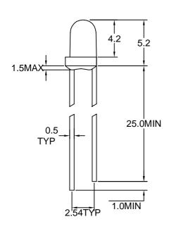
NOTE:1.All dimension are In millimeters tolerance Is ±0.25 unless otherwise noted 2.Specifications are subject to change without notice
